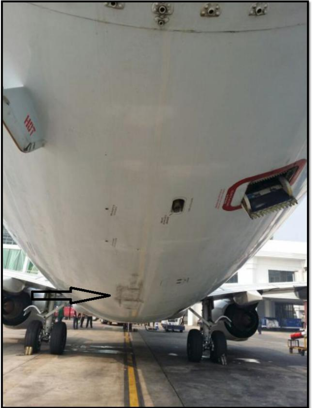
Damage to Belly of aircraft
