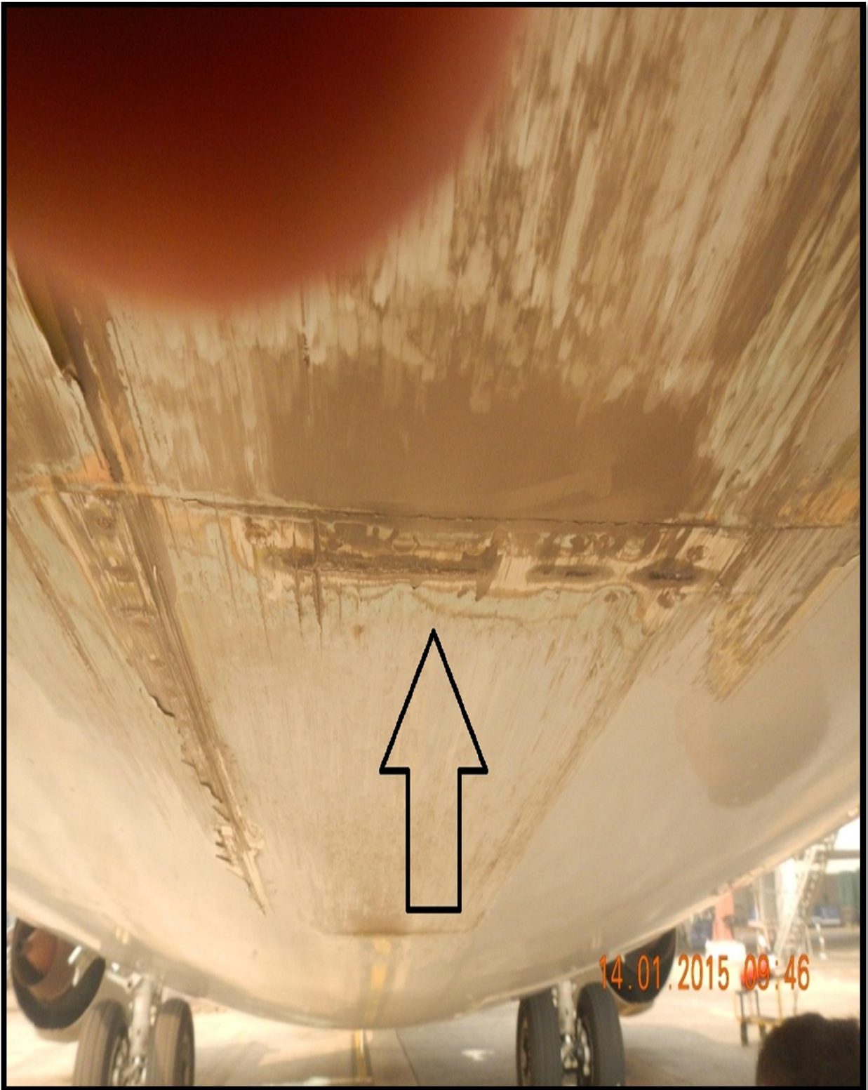
Damage to Belly of aircraft
